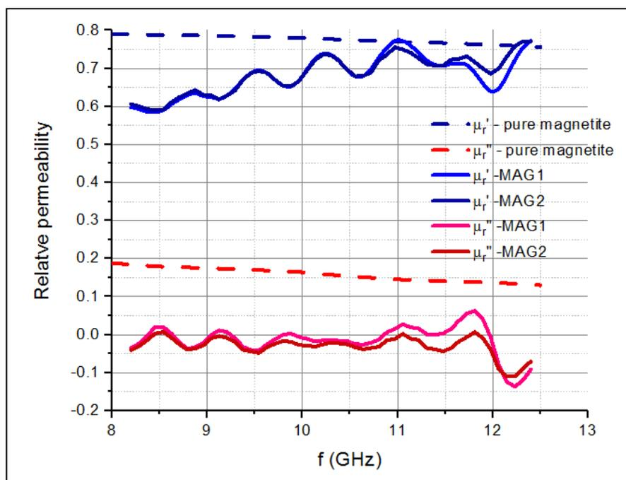
Figure 5. The real and imaginary part of relative permeability of magnetosomes suspensions MAG1 and MAG2 in the SHF range compared to published data on pure magnetite nanoparticles by Kong et al.
