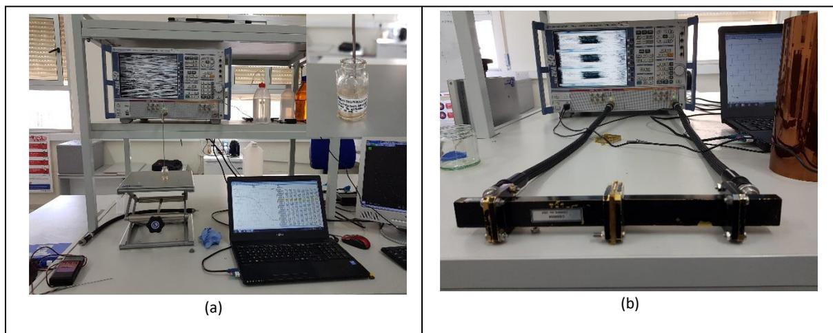
Figure 1. The two experimental setups used to measure the dielectric properties. (a) depicts the reflection method using an open-ended coaxial probe whilst (b) shows the transmission measurement system using a rectangular waveguide – which allows also measurement of magnetic properties.
