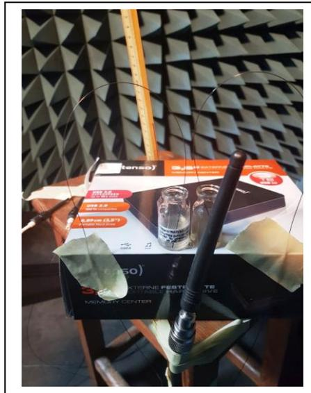
Figure 2. Monopole antenna fed at 4W/440 MHz and magnetosomes suspensions in the near field with inserted optic thermal probes to measure heating during exposure, inside the anechoic chamber.
