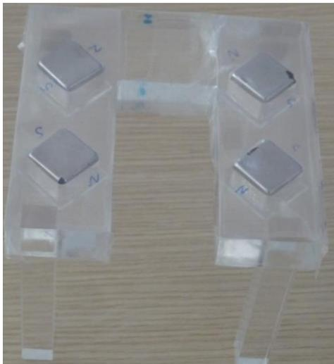
Fig.2. A simple device for focused hyperthermia. The magnets in the diagonals are oppositely polarized
