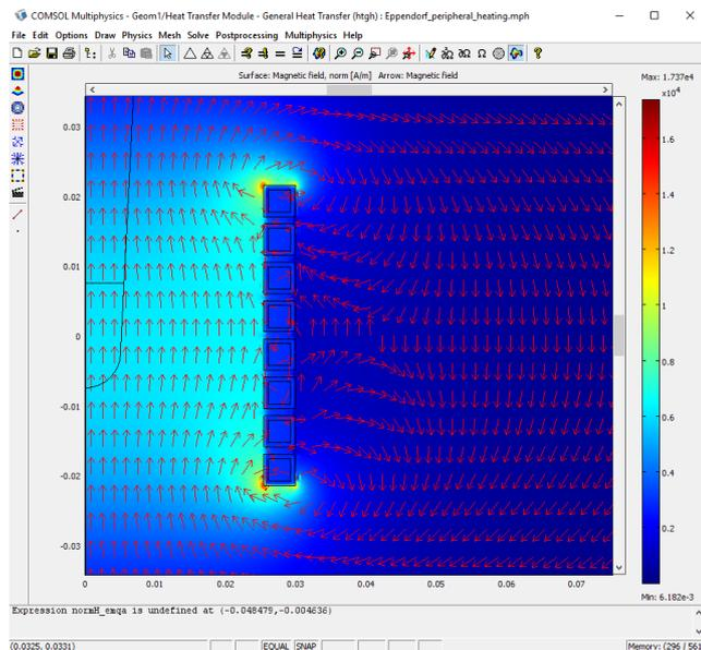
Fig. 3. Magnetic flux density height and direction of one of the coils
