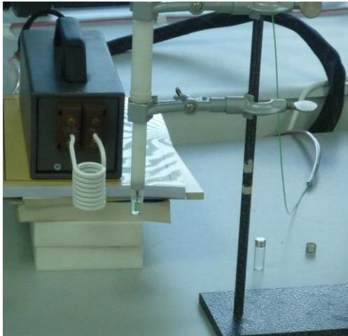
Fig. 1. The resonator (a) and the fiber thermometer (b)
