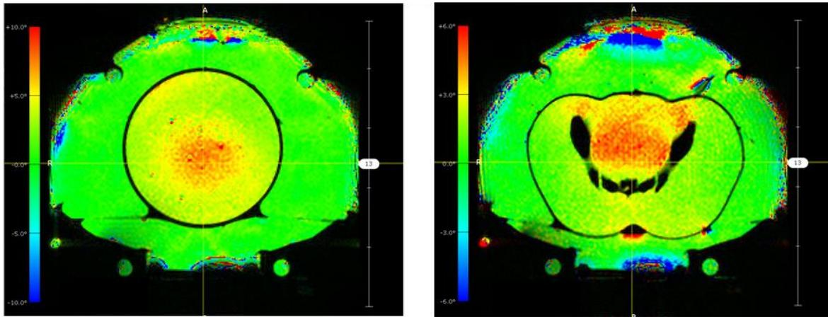
Figure 2. Magnetic resonance thermometry after 11 minutes of heating for central target with 1000W applied power for the cylindrical phantom (left) and 600W applied power for the anthropomorphic phantom (right).
