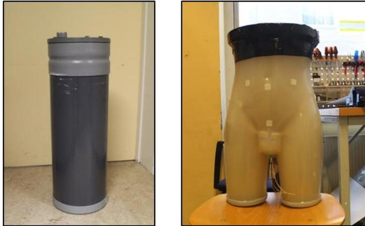
Figure 1. Cylindrical homogeneous phantom (left) and human-shape anthropomorphic phantom (right).
