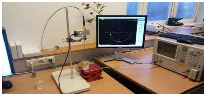
Figure 1: Experimental set-up for dielectric measurement
