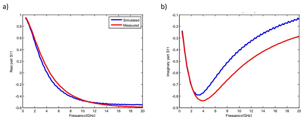
Figure 11: a) Real and b) imaginary part of DI water S11 parameters from both the simulation and the dielectric measurement.
