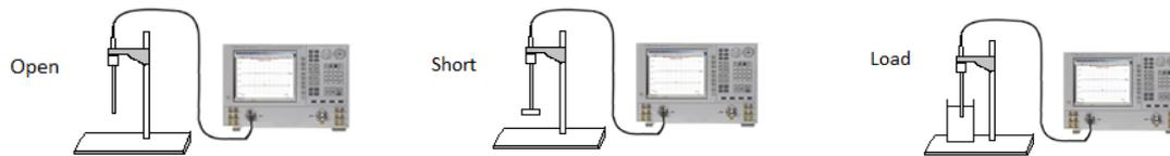
Figure 3: Illustration of the three standard calibration performed by the dielectric measurement of open, short, and load (DI water).
