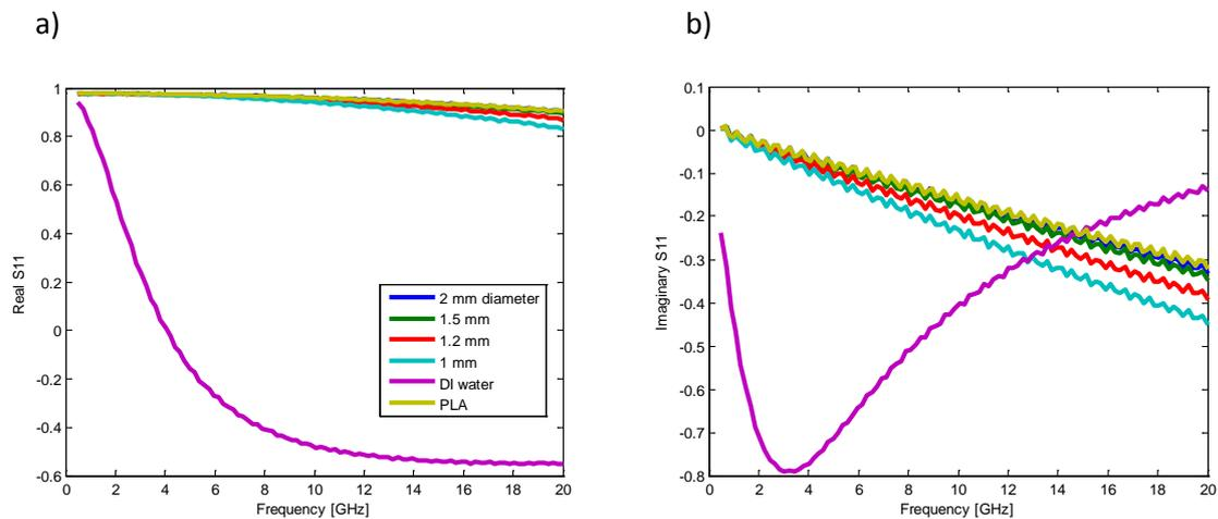
Figure 12: a) Real and b) imaginary part of S11 parameters obtained from the four heterogeneous scenarios and compared to the DI water and PLA simulation parameters.
