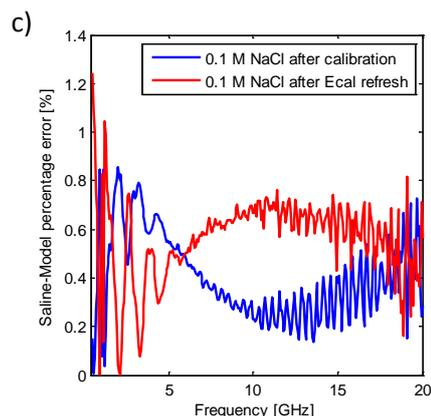
Figure 7: Comparison of the 0.1 M NaCl dielectric data acquired with the slim form probe after the system calibration, after the system perturbation, and after the calibration refresh with ECal in: a) relative permittivity and b) conductivity plots. The acquired data was also compared to the model in [10]. c) For both the measurements performed after the calibration and after the ECal calibration refresh following the system perturbation, the permittivity data accuracy is within 1.3%.
