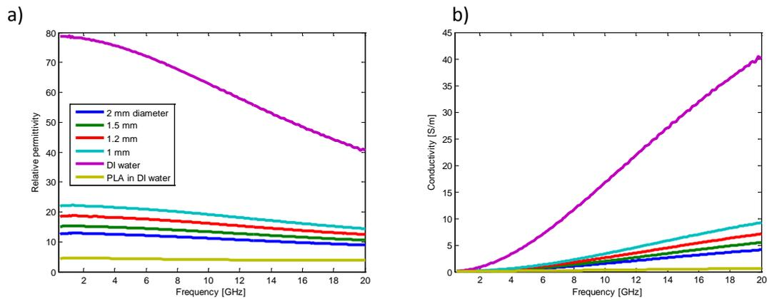
Figure 8: Comparison of the dielectric data from the four samples, DI water and PLA immersed in DI water in terms of: a) relative permittivity and b) conductivity.
