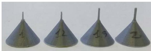
Figure 5: PLA 3D-printed cylinders supported by a conical base and having radii of 0.5 mm, 0.6 mm, 0.75 mm and 1 mm, respectively.
