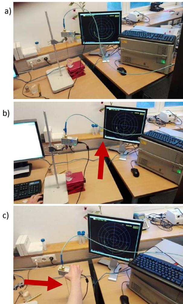
Figure 4: Two examples of system perturbation. a) Dielectric system after calibration; b) Dielectric system after cable movement and position change; c) Dielectric system after ECal position change without the use of the probe holder.
