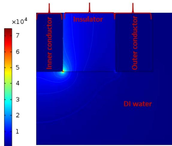
Figure 10: Enlargement the simulated slim form probe tip in DI water. In the simulation a simplified 2D axis-symmetric model was used and the electric field lines propagating from the inner conductor to the outer conductor through the DI water were plotted. Specifically, in this plot, the normal component of the electric field at 2 GHz obtained from simulating the probe in DI water is shown.
