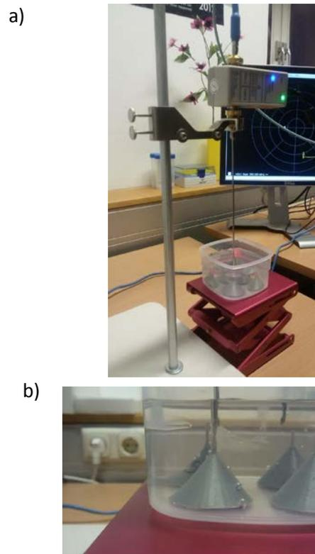
Figure 6: a) Dielectric measurement of the 3D-printed cylinders immersed in DI water. b) Enlargement of the 1 mm radius cylinder in contact with the probe.
