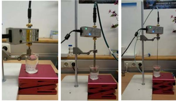
Figure 2: The three probes included in the Keysight dielectric probe kit and used in the experiments: from the left, high temperature probe, performance probe, and slim form probe.
