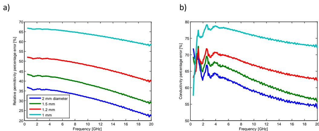
Figure 9: a) Relative permittivity and b) conductivity percentage error between measured dielectric properties and the dielectric properties estimated based on area occupied, from the four radially heterogeneous samples.
