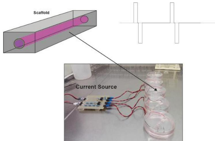
Fig. 1 Schematic of the system for the electrical stimulation of cells in scaffold.
