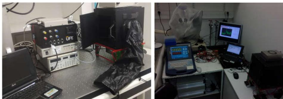
**Fig. 2** Left: Ultra-sensitive luminescence detection system based on selected Hamamatsu H7360-01 photomultiplier and light-tight chamber built in the Institute of Photonics and Electronics, The Czech Academy of Sciences. Right: Combined experimental setup as assembled in France: electric pulse generator (Cliniporator) connected to dark light-tight chamber with luminescence detection.
