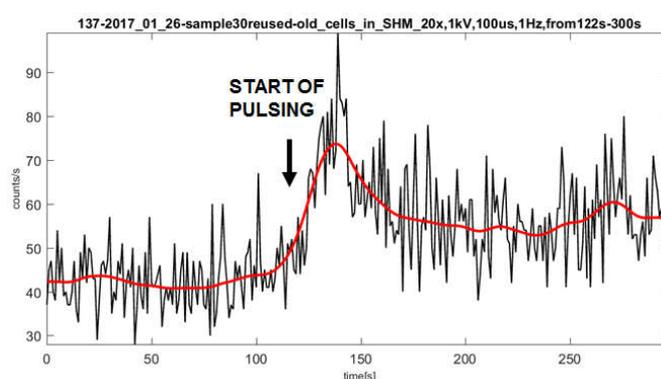
**Fig. 4** Typical chemiluminescence signal from cell suspension undergoing pulsed electric field treatment
