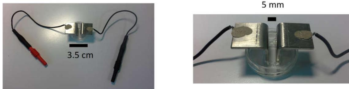
**Fig. 3** The gap between the electrodes used for the experiments was 5 mm. Hence, for example 1kV voltage corresponds to 0.2 MV/m (2 kV/cm) voltage to electrode distance ratio. The sample volume was
