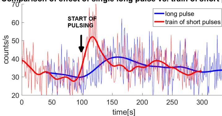
**Fig. 7** Train of pulses (0.2 MV/m 20x 250 us 1Hz - experiment 129) induces stronger response than the single 0.2 MV/m 5 ms pulse (experiment 63).
