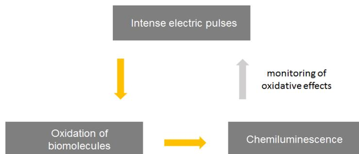
**Fig. 1** Scheme of the principal scientific idea tested during the STSM: Electric pulses induce biomolecule oxidation which in turn causes chemical formation of electron excited states which is manifested as endogenous chemiluminescence. Hence, chemiluminescence can be used to indirectly monitor oxidation of biomolecules in solutions, cells or tissues caused by electric pulses.
