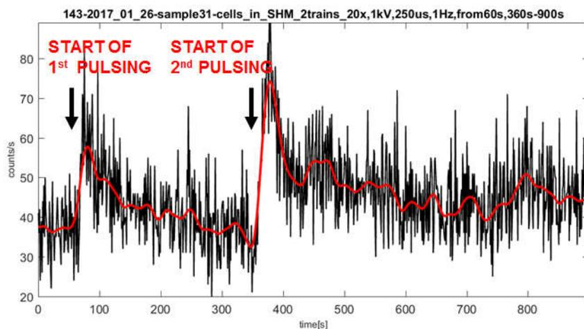
**Fig. 8** The first pulsing primes for stronger response of a following pulsing. Here, 20x pulses 0.2MV/m, 250 us, 1Hz were delivered from 60s and from 360s. Experiment 143, 39 million cells in 0.6 mL SHM medium.
