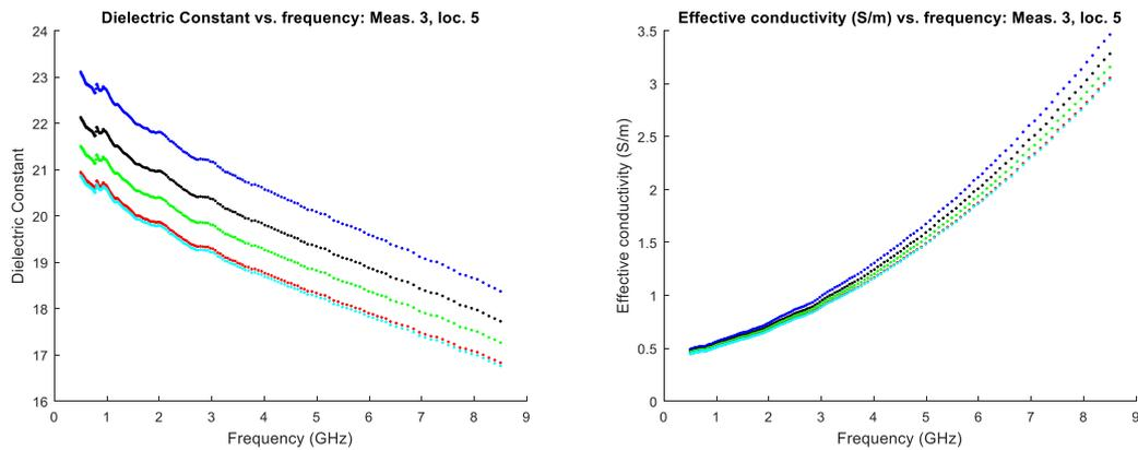
Figure 6. Dielectric constant and effective conductivity of vascularised region in sample 3. Different colours reflect the order of the measurement: blue – 1<sup>st</sup> measurement, black – 2<sup>nd</sup> measurement, green – 3<sup>rd</sup> measurement, red – 4<sup>th</sup> measurement, cyan – 5<sup>th</sup> measurement.
