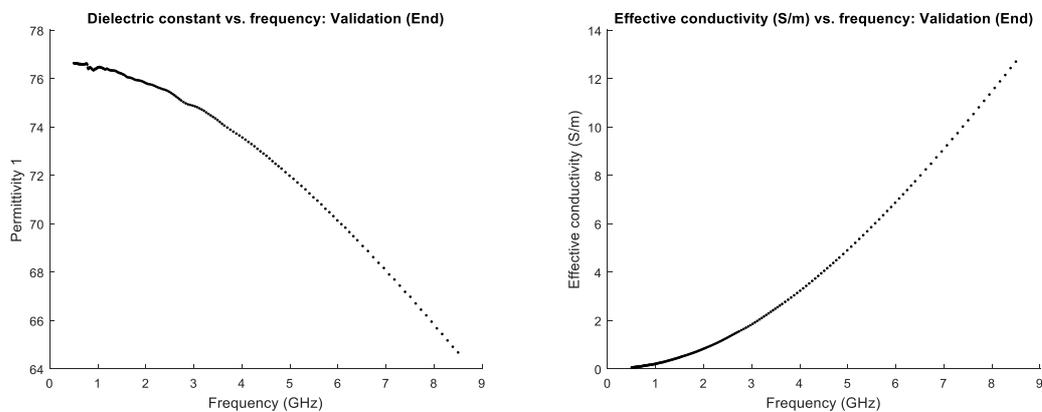
Figure 2. Dielectric constant and effective conductivity of deionised water after the measurement of biological tissue.
