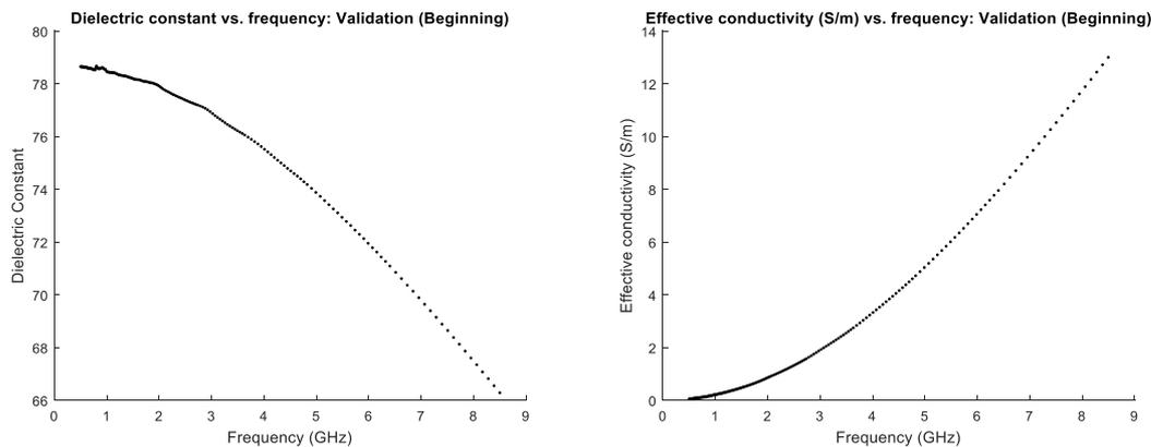
Figure 1. Dielectric constant and effective conductivity of deionised water ahead of measurement of biological tissue.
