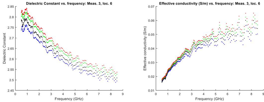
Figure 5. Dielectric constant and effective conductivity of fat tissue in sample 3. Different colours reflect the order of the measurement: blue – 1<sup>st</sup> measurement, black – 2<sup>nd</sup> measurement, green – 3<sup>rd</sup> measurement, red – 4<sup>th</sup> measurement.
