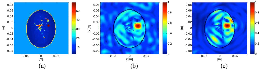
Fig.1 Focusing of vector fields (TE polarization) in a slice of fatty breast: (a) permittivity profile, (c) OCPF [3] focused field intensity, (c) optimized TR [4] focused field intensity.
