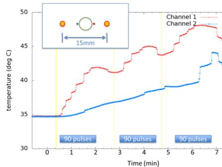
Figure 1: temperature recorded during IRE in two fiber optic thermometry probes positioned around a bile duct in between two IRE electrodes during three pulse trains in a two electrode implant in the pancreas.
