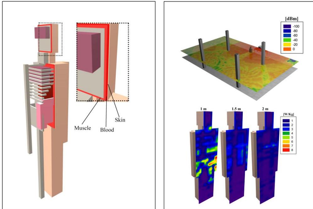
Figure 1: Detail of the Simplified Human Body model implemented and coupled to the 3D Ray Launching Code. Estimations of E-Field values and SAR at human body model surface for an indoor scenario with an operating microwave oven.
